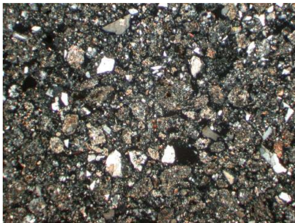
PP08-3365: Representative chips of pervasively muscovite (sericite), quartz-biotite and biotite-sericite aggregate and anhedral quartz grains and aggregates. A) PPL, B) XPL, FOV \approx 4.5 mm.
