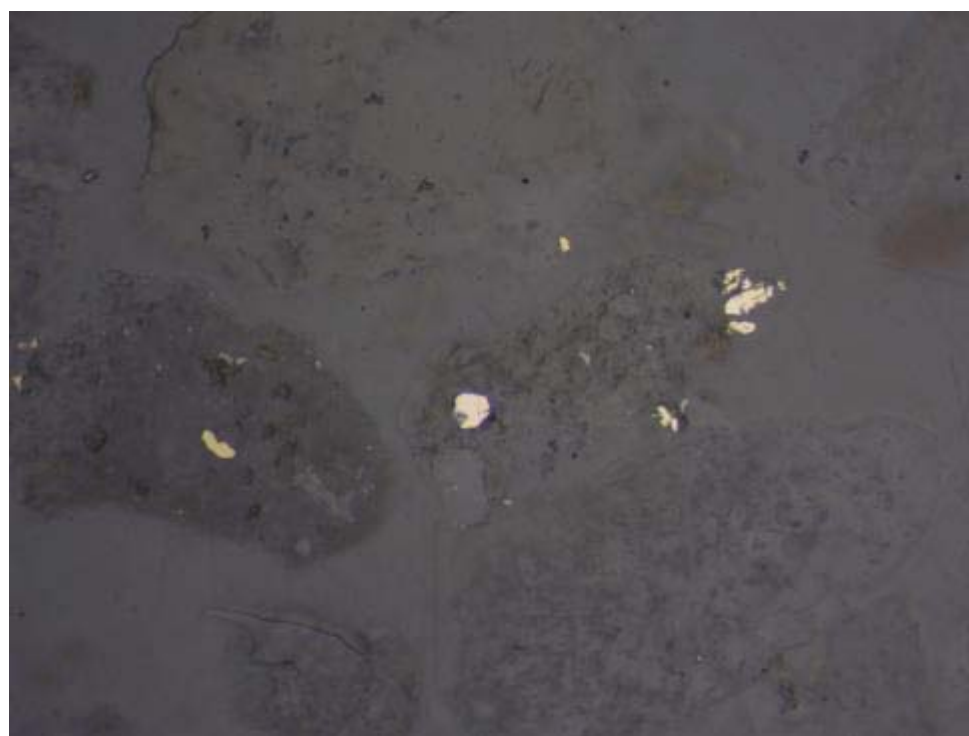
PP08-3850: E) Top: Overview of tailings showing distribution of very fine-grained pyrite and chalcopyrite grains. RL, FOV \approx 2.8 mm. F) Bottom: Anhedrall pyrite grains (centre and right) with irregular boundaries but no alteration rims. Anhedrall chalcopyrite grain (left). RL, FOV = \sim 0.7 mm
