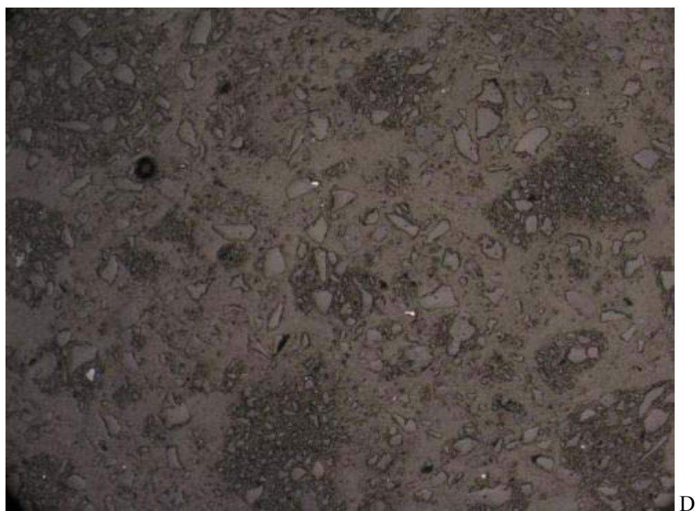
PP08-3610: C) Top, Three liberated colourless carbonate grains. XPL, FOV \approx 0.7 mm, D) Bottom: Overview of tailings showing distribution of very fine-grained pyrite grains. RL, FOV = 2.8 mm
