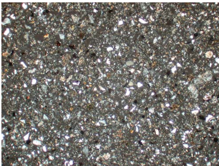
CEMI-20: General view of powder. A) PPL, B) XPL, FOV~ 4.5 mm.
