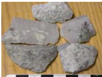
Etched and stained section offcut; scale in cm View of some of the core sample pieces (wet)
