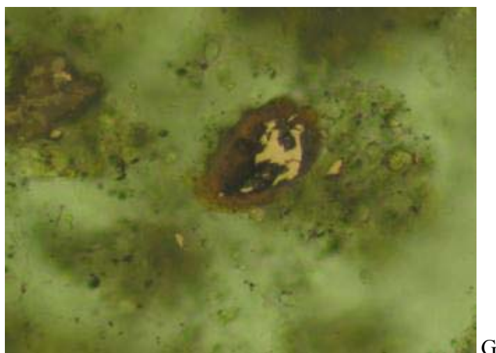
0441-11840-003 Hypogene Pyrite Tail-B: G) Unknown white high reflectance mineral partly replaced by very fine-grained red-brown Fe- oxide/oxyhydroxide aggregates. PPL+RL, FOV \approx 0.1 mm.
