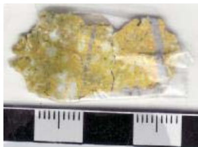
Etched and stained section offcut; scale in cm View of some of the core sample pieces (wet)
