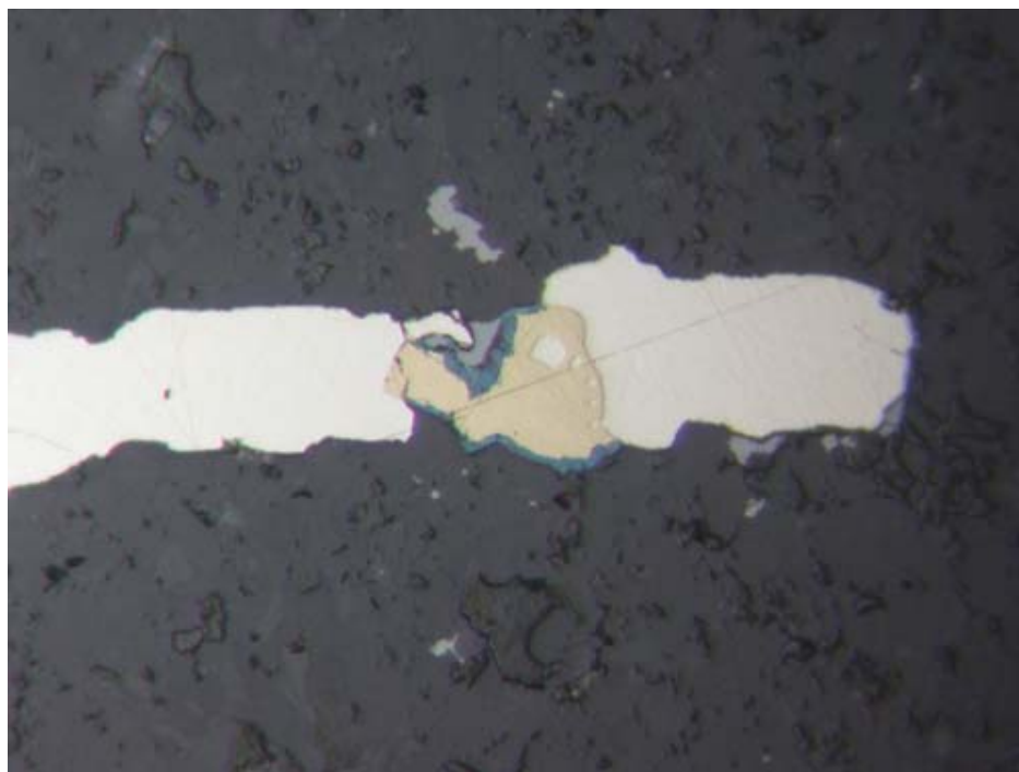
CEMI-18: E) Top, disseminated and fracture-controlled pyrite with inclusions of chalcopyrite and chalcopyrite rimmed by digenite and covellite. RL, FOV \approx 1.1 mm, F) Bottom, pyrite-chalcopyrite-quartz veinlet with chalcopyrite rimmed by covellite. Gray mineral is rutile. RL, FOV \approx 0.3 mm.
