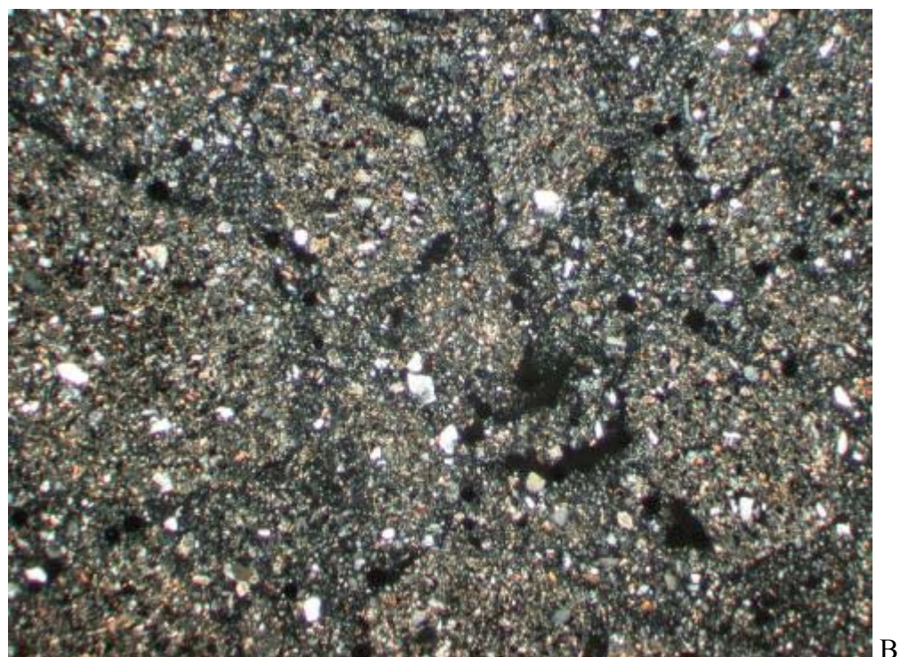
PP08-3607: General view of very fine-grained biotite, muscovite (sericite), quartz grains and aggregates and clumping powder. A) PPL, B) XPL, FOV \approx 4.5 mm.
