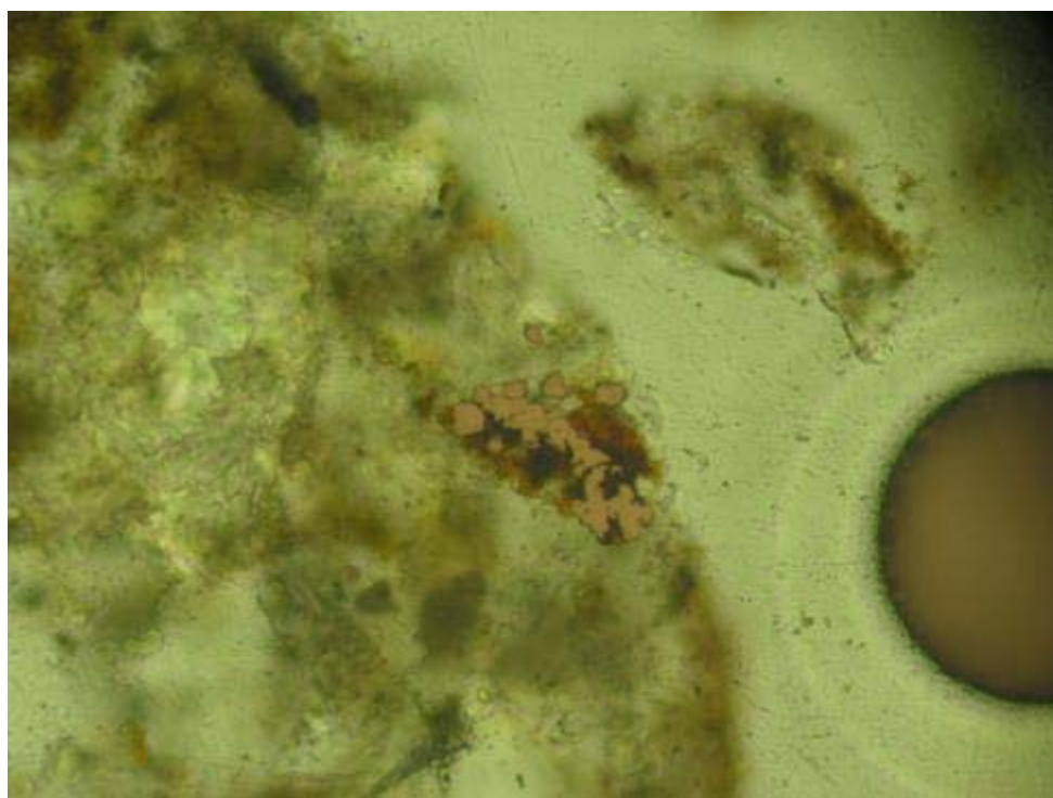
ARLB-007: G) Top: Liberated aggregate of red-brown Fe-oxide/oxyhydroxide with traces of relict pyrite (right), pyrite grain without alteration rims (left of centre). RL+PPL, FOV \approx 0.7 mm. H) Bottom: Very fine-grained pyrite aggregate partly replaced by hematite within granule conglomerate fragment. RL+PPL, FOV \approx 0.1 mm
