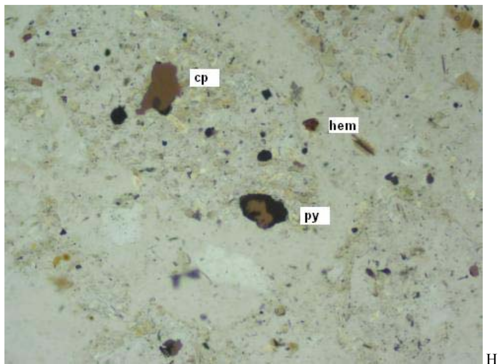
PP08-3365: G) Top: Grain of ?unknown rimmed and virtually replaced by hematite. PPL+RL, FOV \approx 0.1 mm, H) Bottom: Disseminated grains of chalcopyrite (cp), hematite (hem) and pyrite (py). Note black rim around pyrite grain- possibly alteration material plucked from section. PPL+RL, FOV \approx 0.35 mm.
