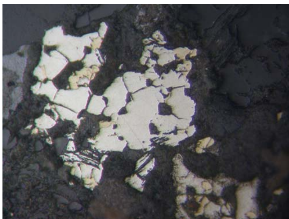
CEMI-15: E) Top, liberated fragment of fine-grained colourless and very fine-grained brown carbonate. XPL, FOV \approx 0.8 mm, F) Bottom, pitted and fractured pyrite and chalcopyrite with black rims. RL, FOV \approx 0.35 mm.
