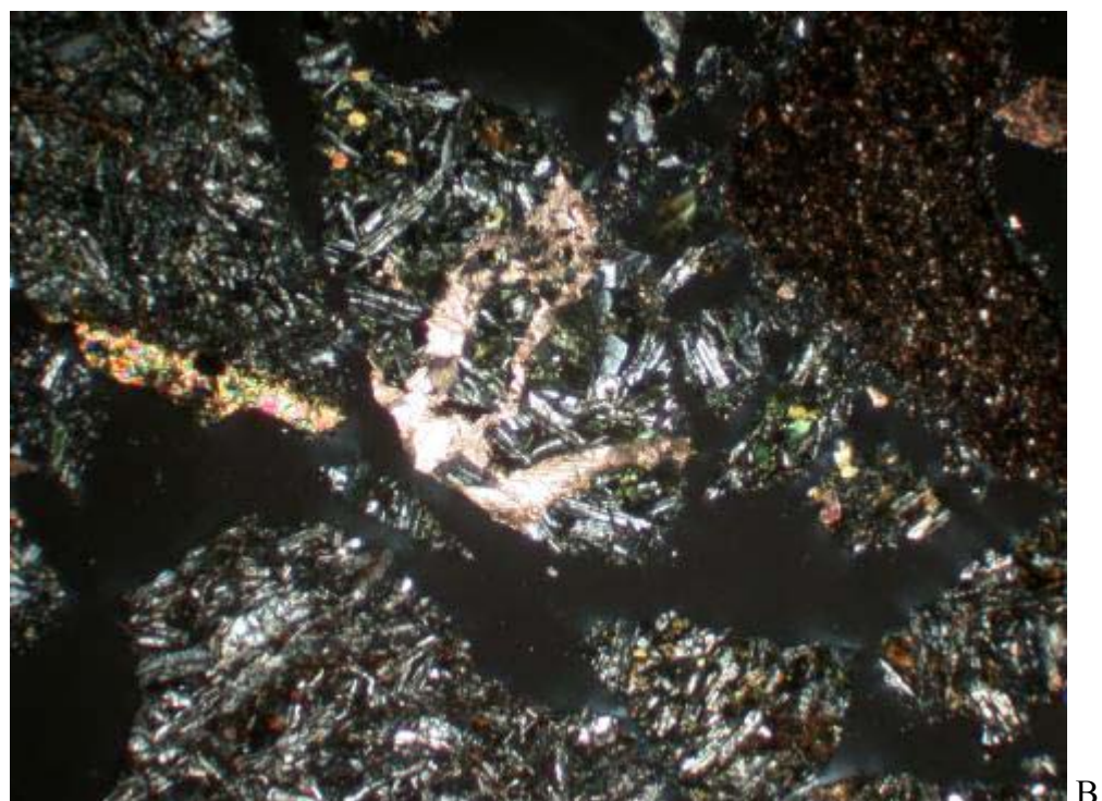
226785: A & B) General view of seriate-textured basalt fragments and siltstone fragment (top right). Note epidote veinlet (far left) and carbonate veinlets (centre). A) PPL, B) XPL. FOV \approx 4.5 mm.
