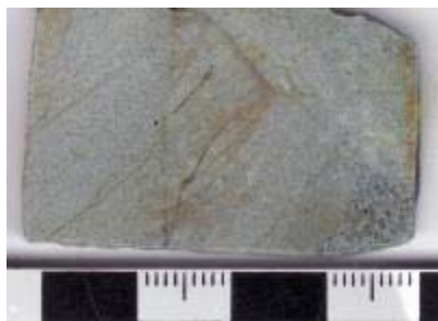
Etched and stained section offcut; scale in cm
