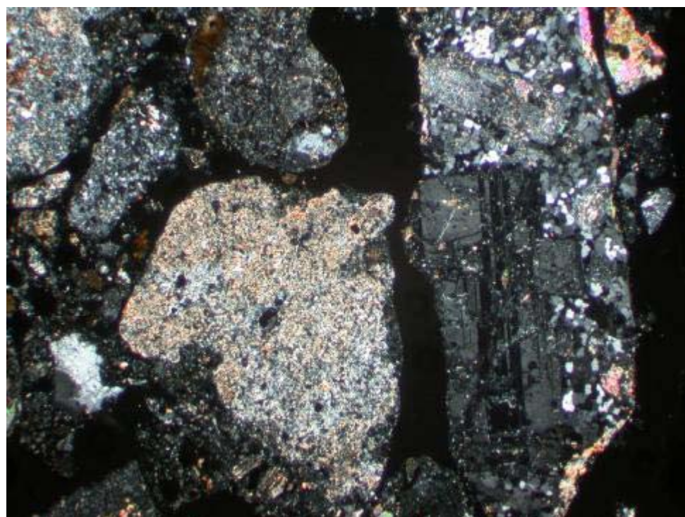
ARLB-006: Representative chips of A) selectively biotite and muscovite (sericite) altered porphyritic rock chips and B) pervasively muscovite (sericite) altered rock (centre) and quartz-feldspar porphyry cut by carbonate veinlet (right). Note liberated carbonate aggregate (top right). XPL, FOV \approx 4.5 mm.
