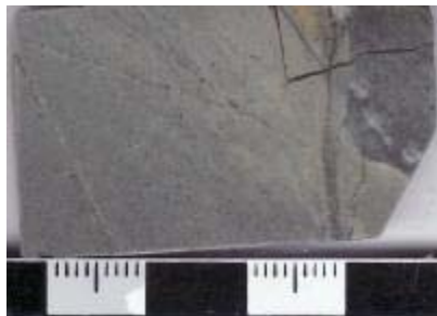
Etched and stained section offcut; scale in cm
