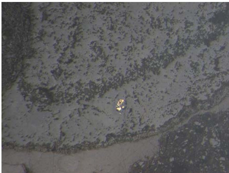
3129-0417-0435: E) Top, Pitted pyrite grains partly replaced by hematite. RL, FOV \approx 0.25mm, F) Bottom, anhedral chalcopyrite within carbonate amygdale. RL, FOV \approx 1.1mm.
