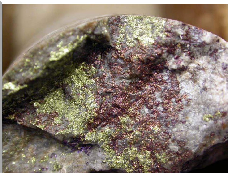
Figure 9.1.4 Core Photo Showing Chalcopyrite and Bornite Mineralization
