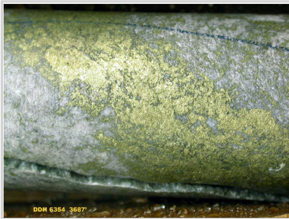
Figure 9.1.5 Core Photo Showing Chalcopyrite Mineralization
