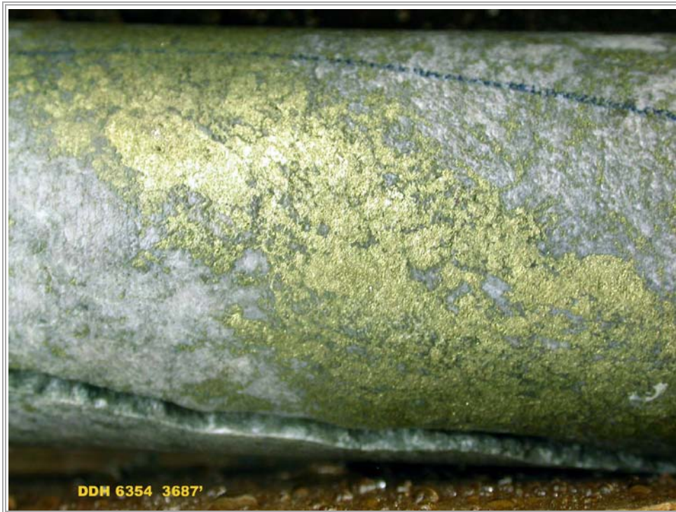
Figure 9.1.5 Core Photo Showing Chalcopyrite Mineralization
