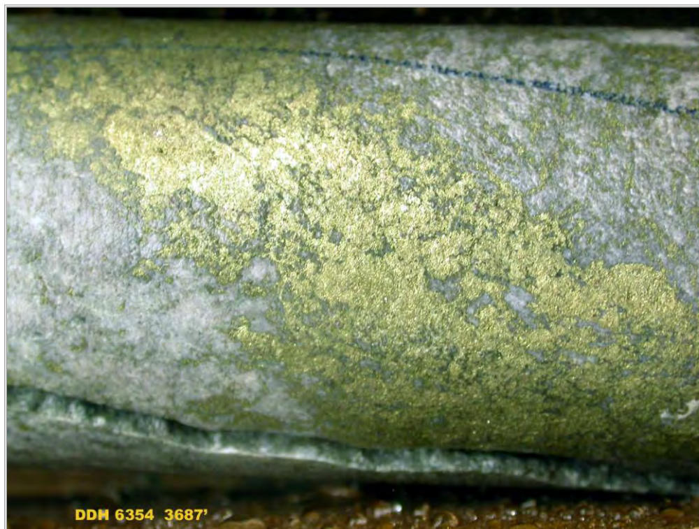
Figure 7.5-1 Drill Core Photograph Showing Chalcopyrite Mineralization
